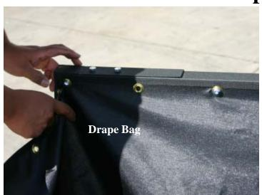
Layout Nylon Drape Bag inside lower opening in assembled frame. Attach 5/16" Button head bolts in appropriate predrilled and tapped holes. (Note: there may be more gussets in bag than holes in frame.)
